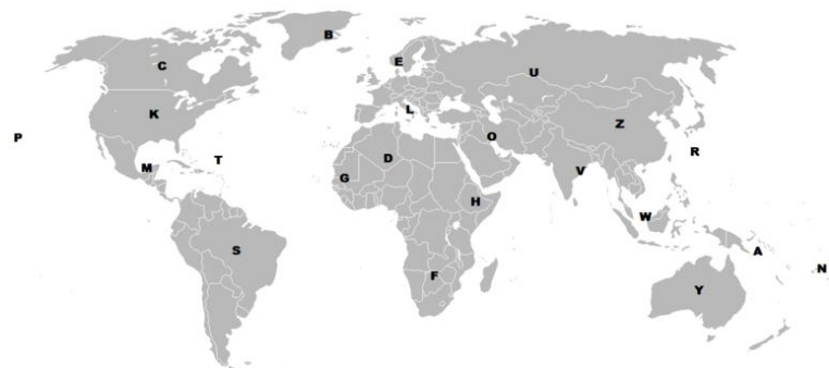
Map of world regions classified according to the first letter of the ICAO airport code. (Indonesia is "W")
